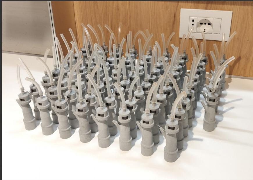
**Figure 3:** Emergency valves for respirators, 3-D printed by Cristian Fracassi and Massimo Temporelli for the Chiari Hospital in Brescia.
